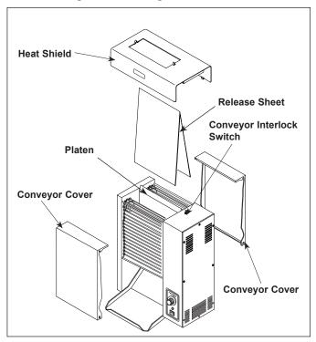
Figure 4. Installing Release Sheet
